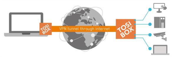
TOSIBOX® solution creates a direct point-to-point VPN tunnel between you and your device. The solution consists of modular components that offer unlimited expandability and flexibility. All components are compatible with each other as well as internet connection, operator, and device agnostic. The solution works both in internal and external networks, and you can connect both modern IoT devices and legacy systems.
